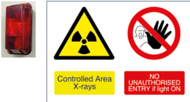
Figure 2.5 Example of a single-stage unlabelled warning light that illuminates automatically when the X-ray set is in a state of readiness to emit X-rays, with a suitably worded accompanying notice
