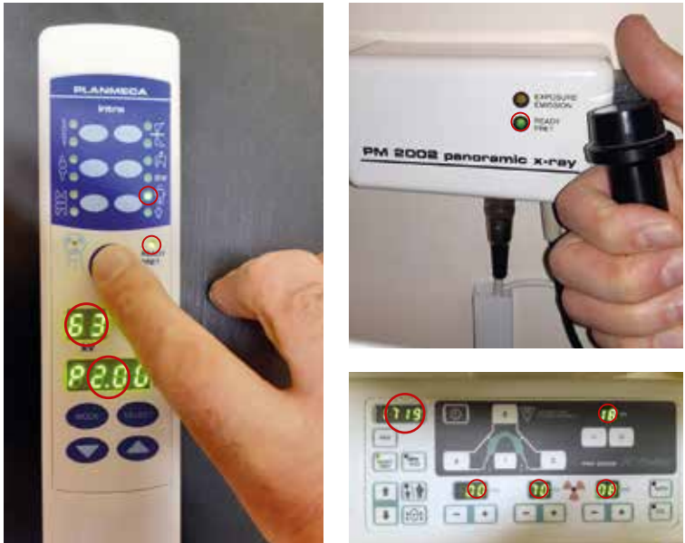
Figure 2.1: Examples of X-ray equipment warning devices with a suitable 'power on' indication (circled in red)
